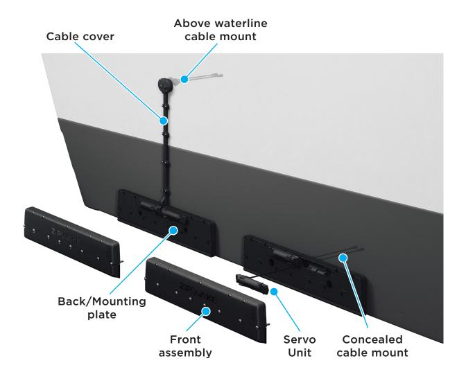
For best effect, different size interceptors can be combined to span as much of the transom edge as possible. A full beam is always the optimal arrangement from a lift-to-drag ratio point of view.
