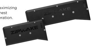
Chine interceptors are particularly useful when transom space is limited abeam of swim platform lifts, waterjets, surface drives, or outboards.
